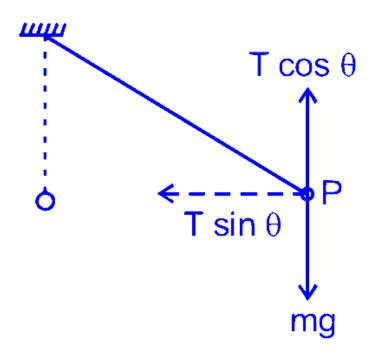
Net force  $= T \sin \theta$  along  $\overrightarrow{PO} \Rightarrow$  Torque about O is zero.
