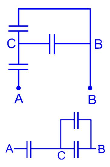
$C_{\text{eq}} = C \text{ series } (C||C) = \frac{2C}{3}$
