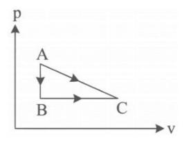
A given quantity of gas is taken from A to C in two ways; a) directly from  $A \rightarrow C$  along a straight line and b ) in two steps, from  $A \rightarrow B$  and then from  $B \rightarrow C$ . Work done and heat absorbed along the direct path  $A \rightarrow C$  is 200J and 280J respectively.
