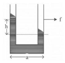
As shown in the figure, a liquid is at same levels in two arms of a U-tube of uniform cross-section when at rest. If the U-tube moves with an acceleration 'f 'towards right, the difference between liquid heights between two arms of the U tube will be, (acceleration due to gravity = g)
