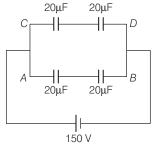
In the branch *AB*, both capacitor are arranged in the series combination. Hence, its equivalent capacitance is given by
