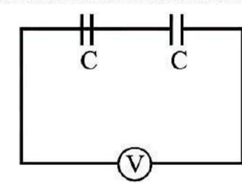
When dielectric is inserted in one of the capacitor,
