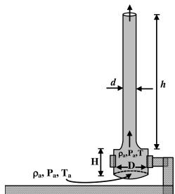
17. When the chimney is closed using a cap at the top, a pressure difference  $\Delta P$  develops between the top and the bottom surfaces of the cap. If the changes in the temperature and density of the hot air, due to the stoppage of air flow, are negligible then the value of  $\Delta P$  is \_\_\_\_\_ Nm<sup>-2</sup>.
