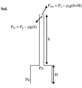
$$\begin{split} P &= \text{constant} \\ \Rightarrow \rho_a T_a &= \rho T \\ 1.2 \times 300 &= \rho \times 360 \\ \rho &= 1 \text{ kg/m}^3 \\ \Delta P &= \rho_a g \ (h + H) - \rho g h \\ &= 1.2 \times 10 \times 10 - 1 \times 10 \times 9 \\ &= 120 - 90 = 30 \text{ N/m}^2 \end{split}$$
