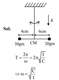
Where I = moment of inertia I = (30) (4)<sup>2</sup> + (20) (6)<sup>2</sup> = 1200 gm-cm<sup>2</sup> = 1.2 × 10<sup>-4</sup> kg-m<sup>2</sup>  $\Rightarrow \omega = \sqrt{\frac{1.2 \times 10^{-8}}{1.2 \times 10^{-4}}}$   $\Rightarrow \omega = \sqrt{10^{-4}}$   $\omega = (10^{-2})$  $n \times 10^{-3} = 10^{-2} \Rightarrow n = 10$
