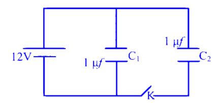
In the figure, first the capacitors are fully charged by closing the key K. Then after opening the Key a dielectric material with dielectric constant 2 is filled in the space between the plates of both the capacitor. At this state the ratio of the Charge on the capacitor  $C_1$  to that of  $C_2$  is:
