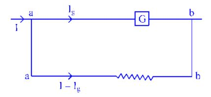
The potential difference,  $V_{ab}=(V_a-V_b)$  is the same for both paths, so  $I_gG=(I-I_g)S$
