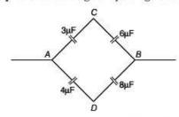
In the upper arm capacitors 3μF and 6μF are connected in series and similarly in lower arm capacitors 4µF and 8µF are connected in series . The equivalent capacitance is given by
