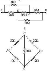
$$\frac{R_{AC}}{R_{AD}} = \frac{R_{BC}}{R_{DB}}$$
