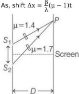
Shift due to one plate  $\Delta x_1(\mu_1 - 1)t$ Shift due to another path  $\Delta x_2 = \frac{\beta}{\lambda}(\mu_2 - 1)t$  Net shift  $\Delta x = \Delta x_2 - \Delta x_1 = \frac{\beta}{\lambda}(\mu_2 - \mu_1)t.....$  (i) Also, it is given that  $\Delta x = 6\beta$ Hence,  $6\beta = \frac{\beta}{\lambda}(\mu_1 - \mu_2)t$  $\Rightarrow t = 6\frac{\lambda}{(\mu_1 - \mu_2)} = 6 \times \frac{4000}{(1.7 - 1.4)} - 80000\text{\AA}$  $\Rightarrow t = 8 \times 10^{-6} = 8\mu\text{m}$
