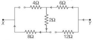
Equivalent resistance between X and Y  $R_{_{eq}}$  = 8 + 2 + 6 =  $16\Omega$
